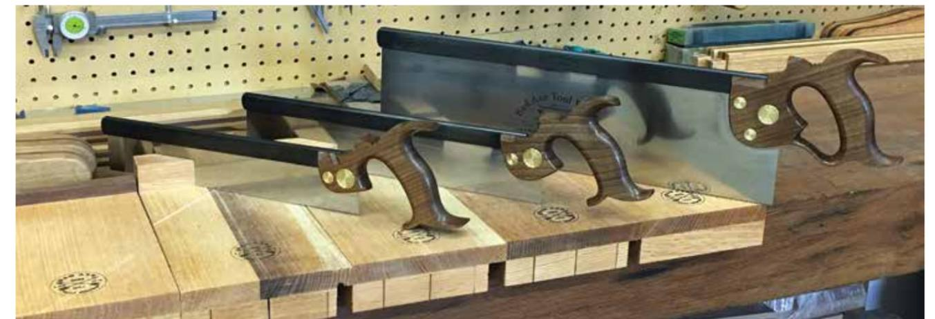
Three steps to workshop heaven: dovetail, carcass and tenon but not necessarily in that order
