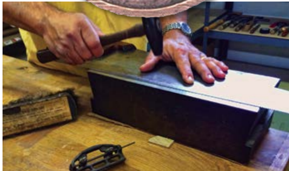
Hammer-smithing a vintage Disston sawplate back into true
