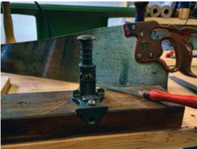
Disston Star hammer saw set, patented 1876
