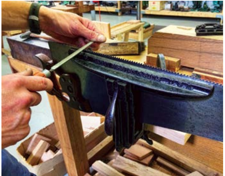
Sharpening a Disston D8 from the 1887–1896 era
