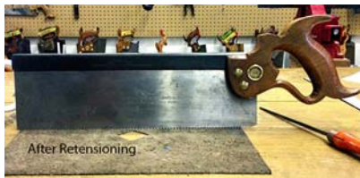
Disston No. 4-12 PHILADA (1896-1917) after retensioning: (plate depth restored to factory setting; sawback now stiffens/straightens toothline)
