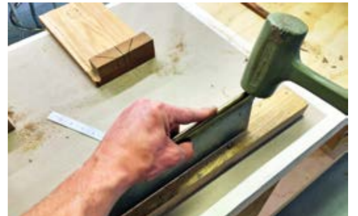
Re-tensioning the toe of a backsaw
