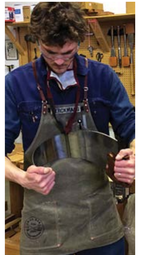
'Flex-testing' a handsaw
