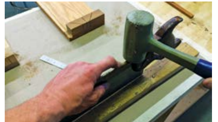
Re-tensioning the heel and the toothline of a backsaw
