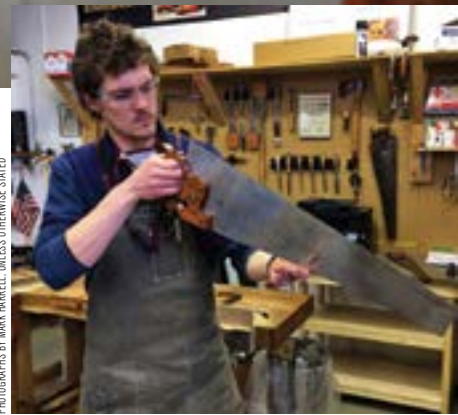
Sighting down the toothline of a handsaw
