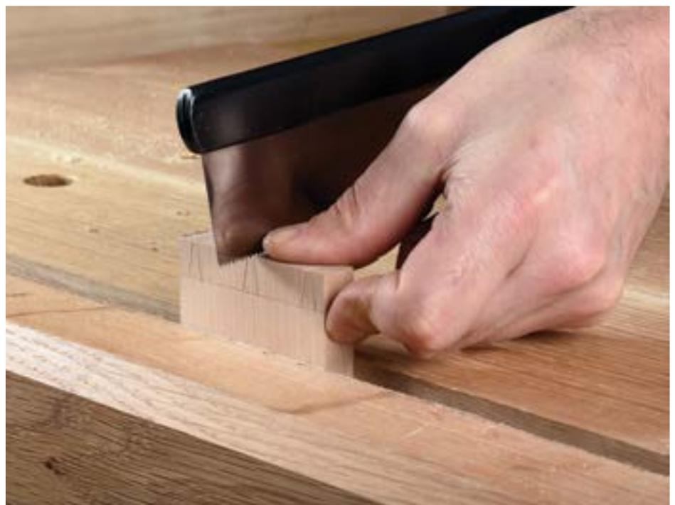
The 015 gauge 300mm-long Bad Axe Stiletto dovetail saw has relaxed tooth geometry at the toe to assist with the start of the cut
